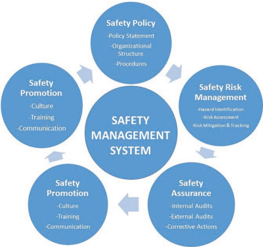
FIGURE 29.1 Components of an SMS.
